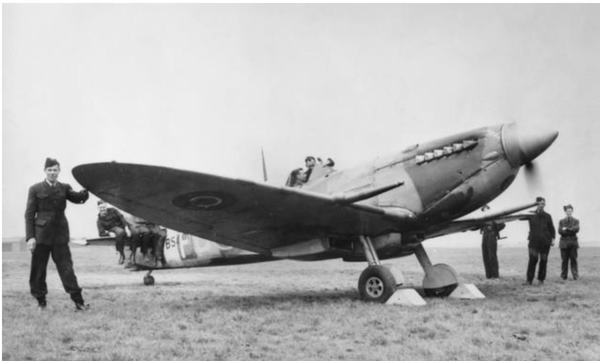
Australian War Memorial photograph UK0090 "Running up" the engine of a Spitfire aircraft before handing it over to the pilot.
