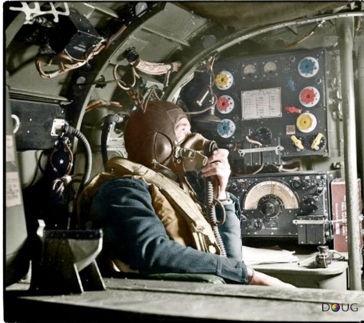
A Wireless Operator in a Lancaster speaking to the pilot from his position in front of the Marconi Transmitter/Receiver set.
