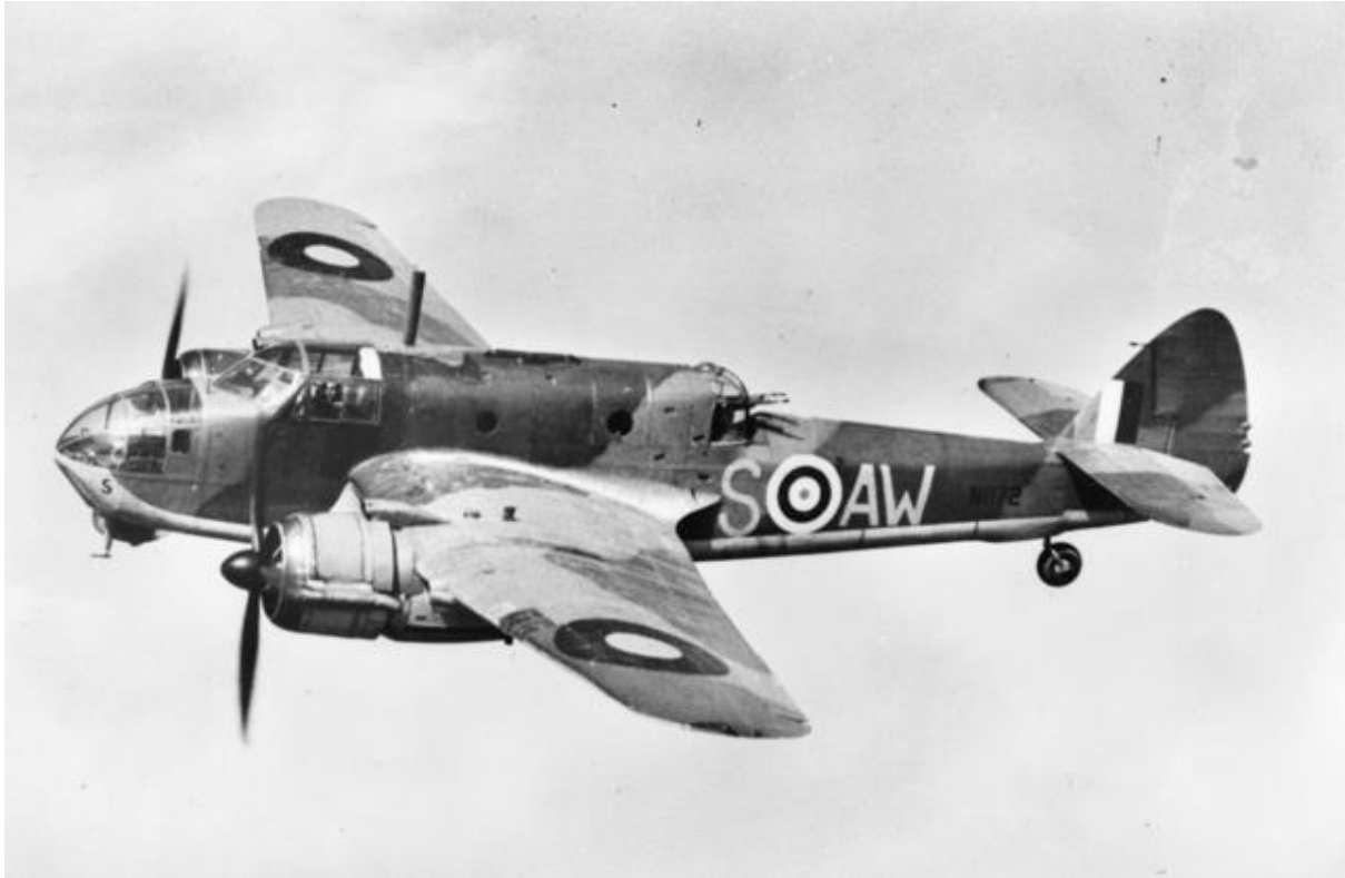
Australian War Memorial photograph 009483 A Bristol Beaufort torpedo-bomber of Coastal Command on patrol duties.
