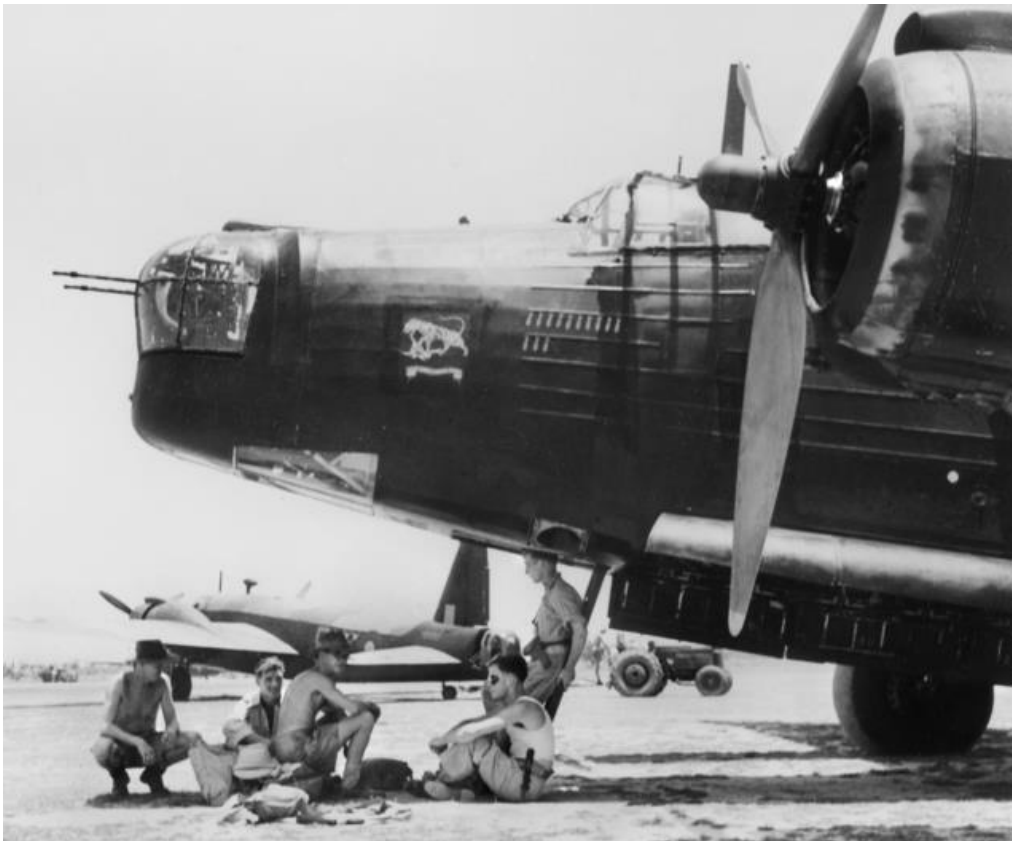
Australian War Memorial photograph SUK12734 Front Air Gunner's position on a Vickers Wellington of the Royal Air Force.
