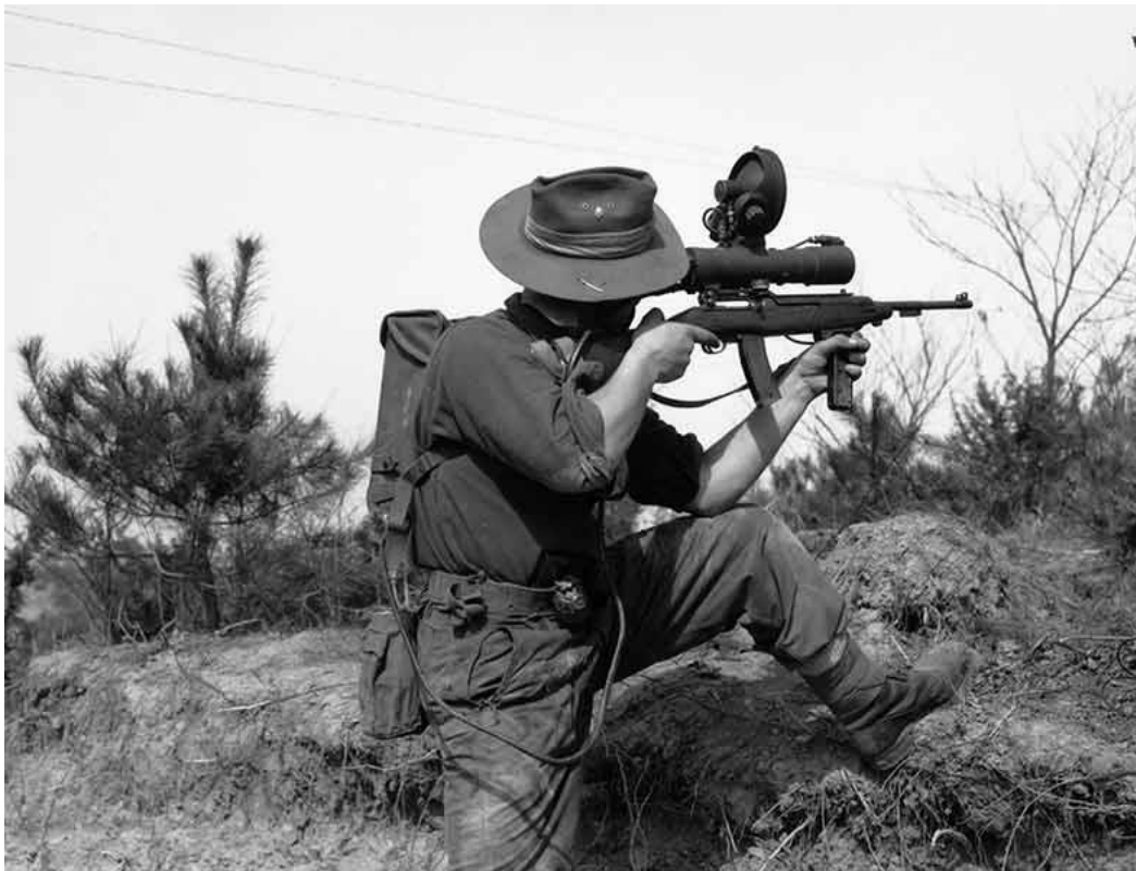
Private L. J. Best of Sniper Section, 3rd Battalion, the Royal Australian Regiment (3RAR), displaying the Sniperscope which is attached to a .30 calibre United States Carbine. The scope is battery operated and the battery is carried in the pack on his back. [AWM 147849]
